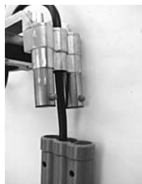
Detaching housing from bracket
