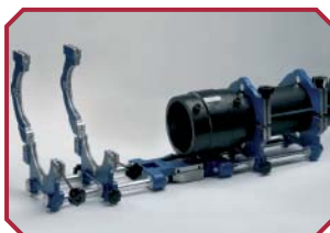
Tighten with the clamping device and slide the socket into the pipe. Never touch the inside or the outside surfaces of the cleaned socket and scrapped pipe ends.
