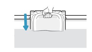
After placing the robot in the water, please wait 2-3 minutes for it to prepare for cleaning. The robot will sink to the pool floor and release the air from the buoyancy chamber, then begin cleaning automatically.
